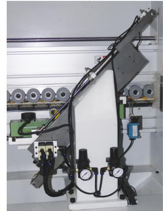
**Heated In-feed Fence, Pneumatic Gap Control**
