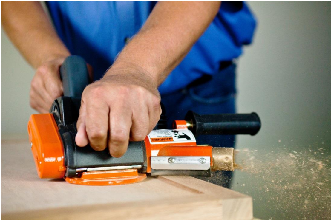
(BH-556 Lipping Planer in operation – dust collection hose removed for clarity)
