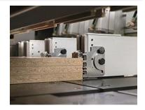
Suction optimization automatic system. All extraction hoods are equipped with pneumatic cut-off valves. The opening/closure of such valves is actuated automatically by the machine depending on the requirement of the cutting pattern. The closure of the valves avoids a useless loss of suction power.
