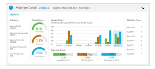
Advanced indicators: indicators specific to the type of machine, with the possibility to select the indicator of interest, the period of analysis and the level of aggregation desired (month, day, hour or half hour).
