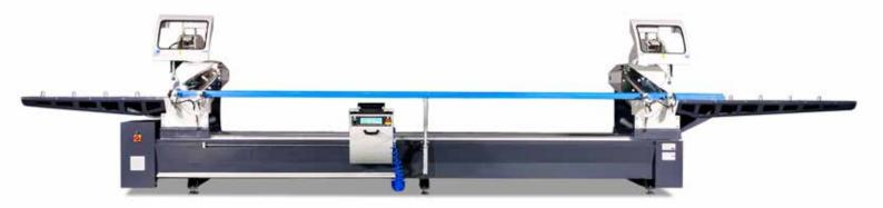
The GEMINI - V R, which is a PLC controlled, Full Automatic Digital Double Head Cutting Machine with Forward Motion Blade of Ø 550 mm, is designed and developed in line with user demands to meet the needs of professional workshop owners and those who are willing to become professionals.
