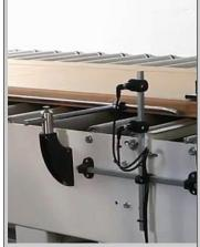
AUTOMATIC READING OF THE BOX DIMENSIONS, to adapt the process to the production requirements, starting from the large-scale to the small dimension batches down to the batch 1 manufacturing.
