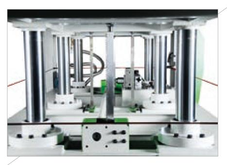
**Synchronised lifting movement** of the 6 cylinders with double rack and pinion arrangement (2 lengthwise 2 widthwise).
