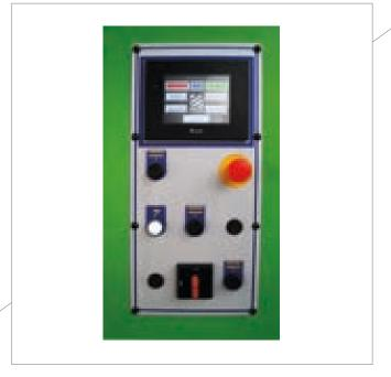
The machine is equipped with a 5.6" PLC Touch screen for easy setting and quick monitoring of the functions.
