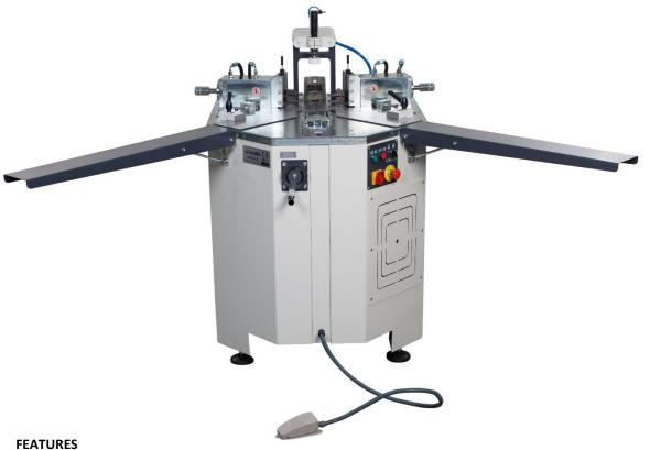
Used for corner crimping processes of aluminum profiles.
