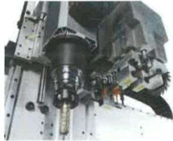
Main routing unit equipped on a cast aluminium sliding support NC managed.
