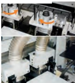
PRE-MILLING UNIT To rectify the edge of the panel prior to banding. (2) 2.5HP HF Motors 2500 rpm, spinning in opposite directions.
