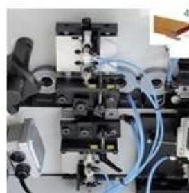
GLUE SCRAPING UNIT Top & Bottom Scraping
