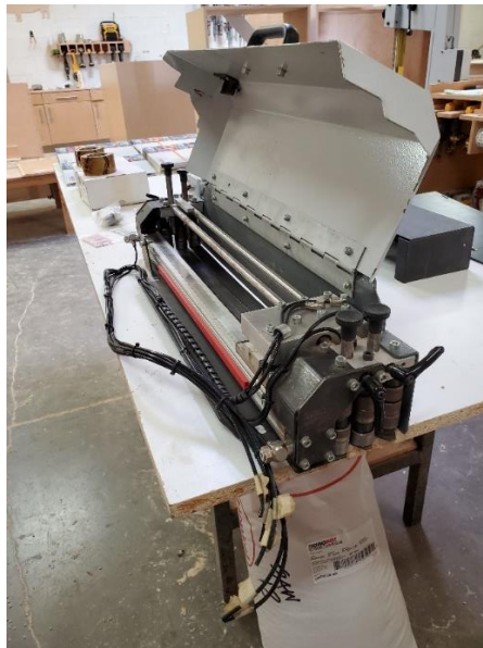
freshly sharpened diamond tipped premill cutters, multi feed unit
