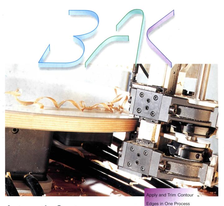
Automatic Contour Edgebanding Machine Optimat BAK 41
