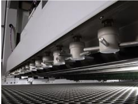
Workpiece blowing off unit - with WEBER ES system energy-saving workpiece controlled workpiece cleaning
