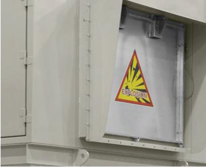
Requirement by NFPA for reactive material such as wood dusts and chips, aluminum and/or magnesium collection.
