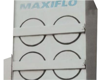
Safety device preventing unauthorized access to cartridges.
