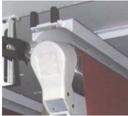
Abrasive Belt Blowers with timer 2 nd and 3 rd working unit. Q6000520, Q6000530
