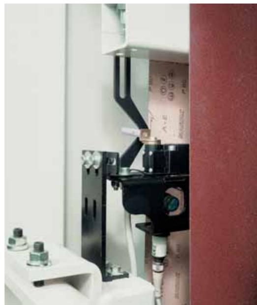
Belt oscillation controlled by an electronic photocell
