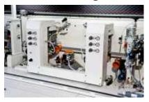
to carry out the front and rear rounding on the transversal side of shaped panels or on PVC/ABS edges and thin solid wood with a very high degree of finishing quality:
