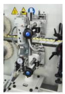
With the heating of PVC/ABS edges it allows the brightening of the colour.
