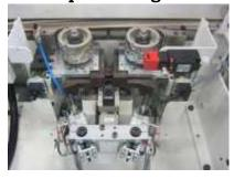
it trims the panel edge obtaining a perfect uniform surface for the glue application and a perfect jointing line with the edge. The unit is equipped with:
