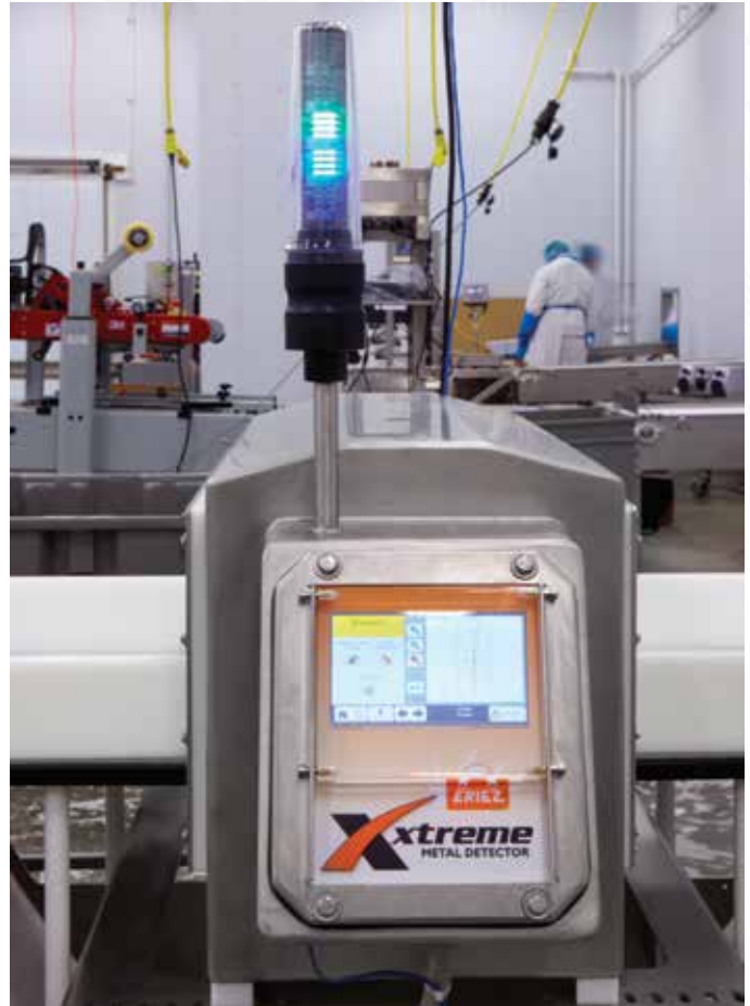
The Xtreme ® Metal Detector pushes the detection/productivity curve with the ability to detect 0.4 mm spheres.
