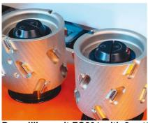
Pre-milling unit FG201 with 2 cutter units
