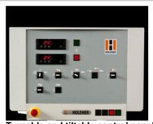
**Turnable and tiltable control panel**, ergonomically located on the inlet side with selector switches for adjusting the units with temperature control for the heating circuits in the adhesive application system
