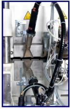
A81576 <u>BUFFING UNIT SPN</u> For the cleaning and finishing of plastic edges: It is composed of two overlapped motors that tilt vertically.
