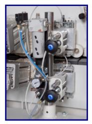
A51706 DOUBLE EDGE BRIGHTENING UNIT PH/1600 This unit brightens colors on PVC/ABS edging with super heated air. The unit receives air from the compressed air distribution system and gives out hot air through two independent nozzles.
