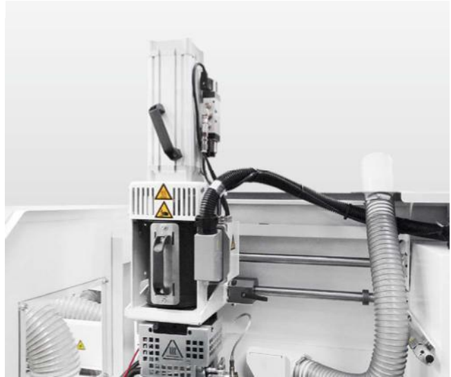
Melting unit in three versions: EVA, PUR as well as EVA and PUR ▪ Efficient processing, as the adhesive is pre-melted ▪ Melting capacity max. 2.5–4 kg/h ▪ With the combination EVA and PUR, it is fast and easy to change the type without cleaning thanks to interchangeable containers
