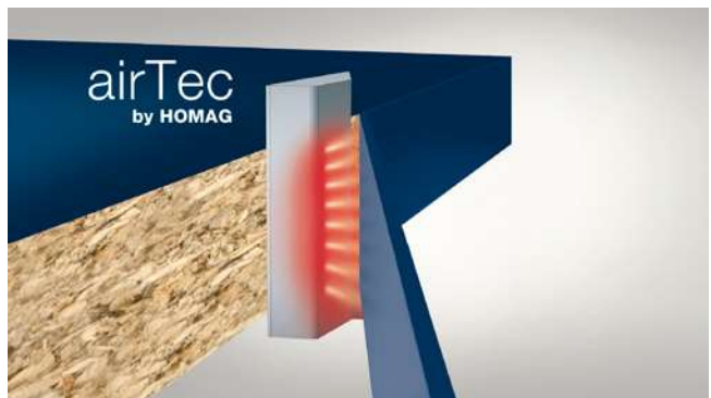
Zero joint technology with HOMAG airTec
