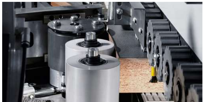
Pressure zone Heavy pressure zone up to an edge thickness of 3 mm and a panel height of 50 mm for optimum glue joint quality (optional: 6 mm edge)
