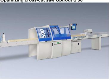
Integrated system consisting of cross-cut saw and motoric positioning pusher for automatic cutting. Quick and reliable cutting of single parts or packets. Inclined machine design in order to allow the alignment of the workpieces at the guide ruler. The heavy, welded saw body as well as the saw aggregate are the basis for precise cuts.
