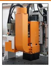
Dust/Chip collection is accomplished with a dust shroud surrounding the main spindle. The dust shroud is connected to the customer supplied dust/chip extraction system through a 6" (152mm) diameter steel adapter.
