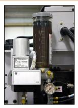
All positioning bearings, ball screws and racks are serviced by an automatic lubrication system, activated directly by the machine control. This ensures the rack and pinion, ball screw and linear guideways are being lubricated to the manufacturer's specifications.
