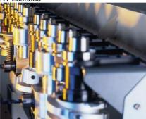
Tool changer 7875, 14-compartment linear pick-up tool changer, pneumatically lifting maximum tool weight: 5 kg per tool or 60 kg total weight
