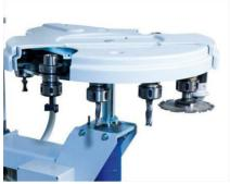
18 position tool changer 7996, (disk) automatically in X-direction following Max. tool Ø: with full equipment Ø 85 mm, with free adjacent spaces Ø 200 mm; saw blades up to Ø 300 mm Max. tool weight: 5 kg per tool or 60 kg when fully equipped with clamping system connector with HSK - shaft
