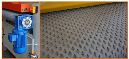
All models come **standard** with a panel mount VFD controlled feed belt allowing the operator total control of speed from 0 to 25 m/min. Heavy-duty 3 ply conveyor belt with automatic belt tracking. Also, available with optional vacuum hold-down for small parts processing.
