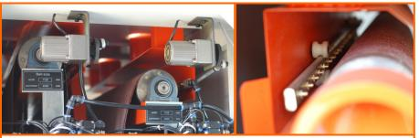
The oscillating integrated air-jet blower with low compressed air consumption is ideal for premium belt cooling and cleaning for a longer belt life and a superior quality finish. Additional vacuum port located on each head.
