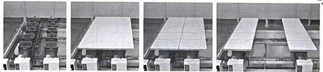
Working table with pods (optional to be added) and rails automatically positioned, which grants the maximum grade of usage easiness and set-up free of mistakes.
