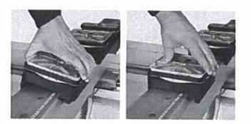
This technology turns into a working table free from vacuum tubes, plugs or connectors and provides the ability to lock even small sized parts simply pairing pods and/or rails to the minimum distance possible.
