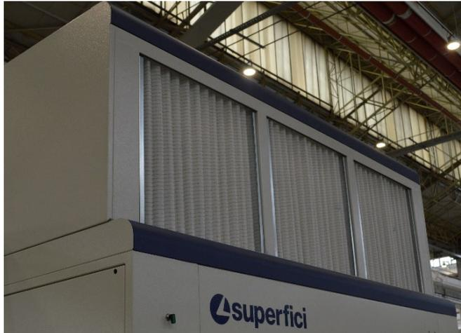
The pressurization system consists of two air intake blowing fans combined with a prefiltering system located on the two sides of the cabin, allowing easy access for inspection, as well as a filtering roof inside the booth.
