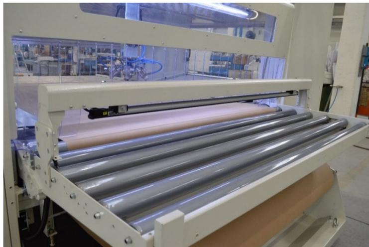
Reading bar as an alternative to the side sensors; a full reading bar across the entire width to identify the spaces between side-by-side panels or any windows.
