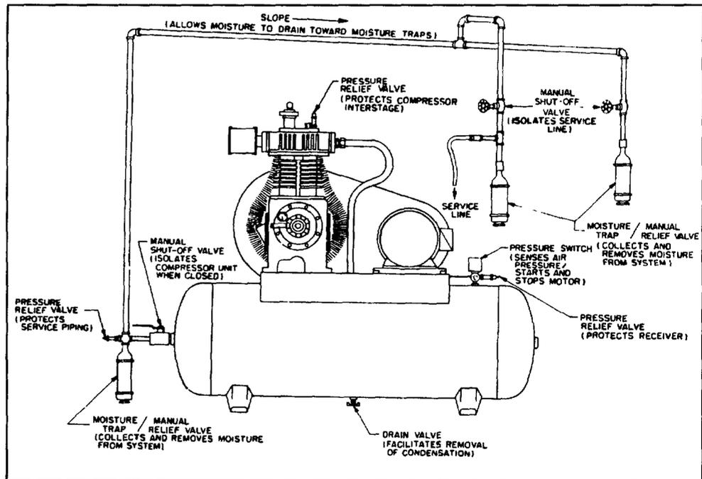
**Fig. 3-1 Typical Drop Leg & Component Location**
