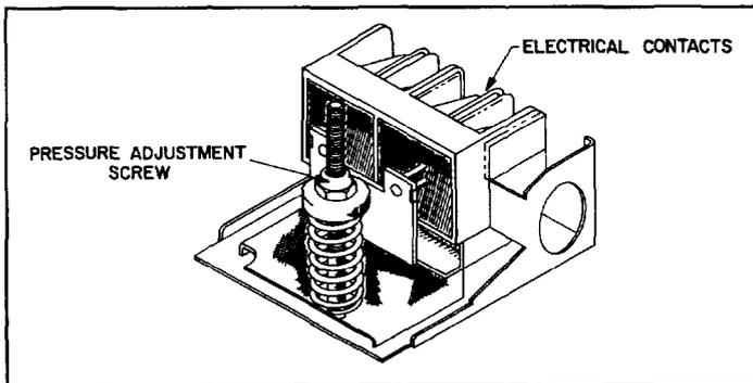
Fig. 5-3 Pressure Switch Pix 1067
