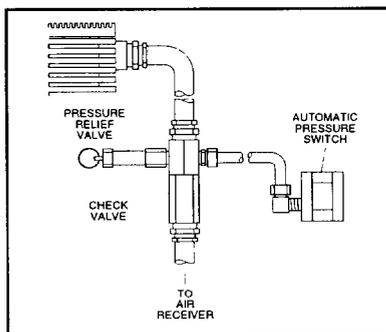
Fig. 2-3 Control Version L Variation (Discharge Line Check Valve & Pressure Switch)
